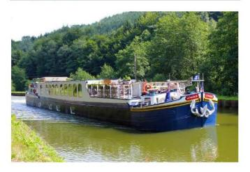
Commercial freight barge Former purpose: Year of construction: 1959 Dimensions: 129ft (39.3m) x 16ft (4.85m) Year converted into a Hotel Barge: 1998 1 x 30 kva and 1 x 40 kva Generators: 1 x 350 CUMMINS Main Engine: Maximum speed: 12 knots Water capacity: 12,000 litres Fuel capacity: 4,000 litres
